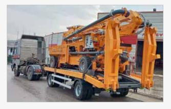
The frame of the FT 208 Trailer can be folded down while being shipped. For overseas shipments, the Scorpion Pump and its carrier trailer can be shipped with the same 40' HC container.
